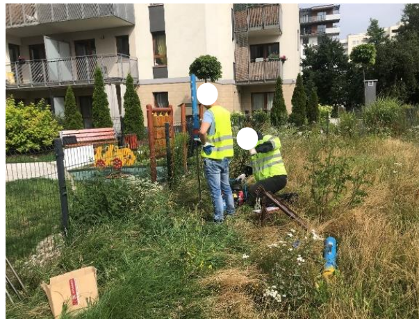
Fig. 4. Overall view of a DPL dynamic probing soil compaction test.
