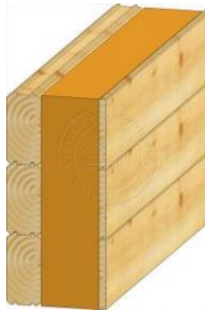
Fig. 3. Insulated log wall, [2].
